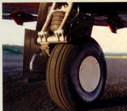
Thanks to those cowl air inlets, CHTs stay under control (top left). New winglets (top right) add a few inches of wingspan and help add knots at altitude. The Acclaim retains many signature Mooney design elements, such as the landing gear's rubber-sleeve (bottom left) and PreciseFlight speed brakes (bottom right).
